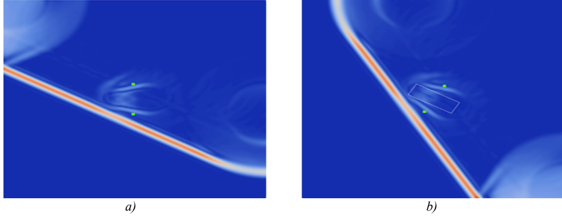
Fig. 2. Wave patterns at one of the time points: a) without using the superimposed grid (the position of the receivers is marked in green); b) using the superimposed grid marked in white, green is receivers
